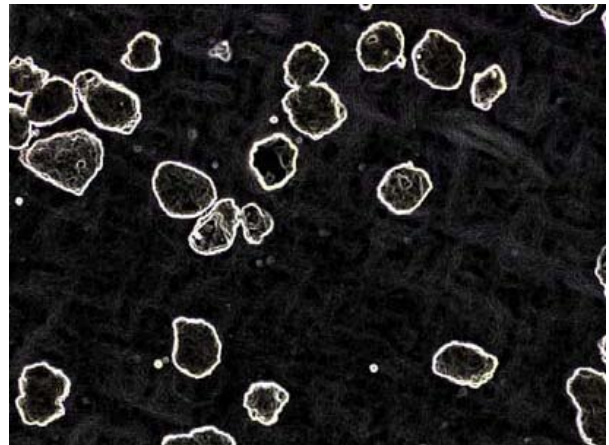
Figure 2: The same field as Figure 1, after edge detection using the Kirsch algorithm.
