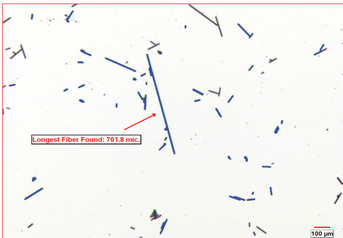
Longest fiber found in current sample. Only the particles appearing in blue were measured.
