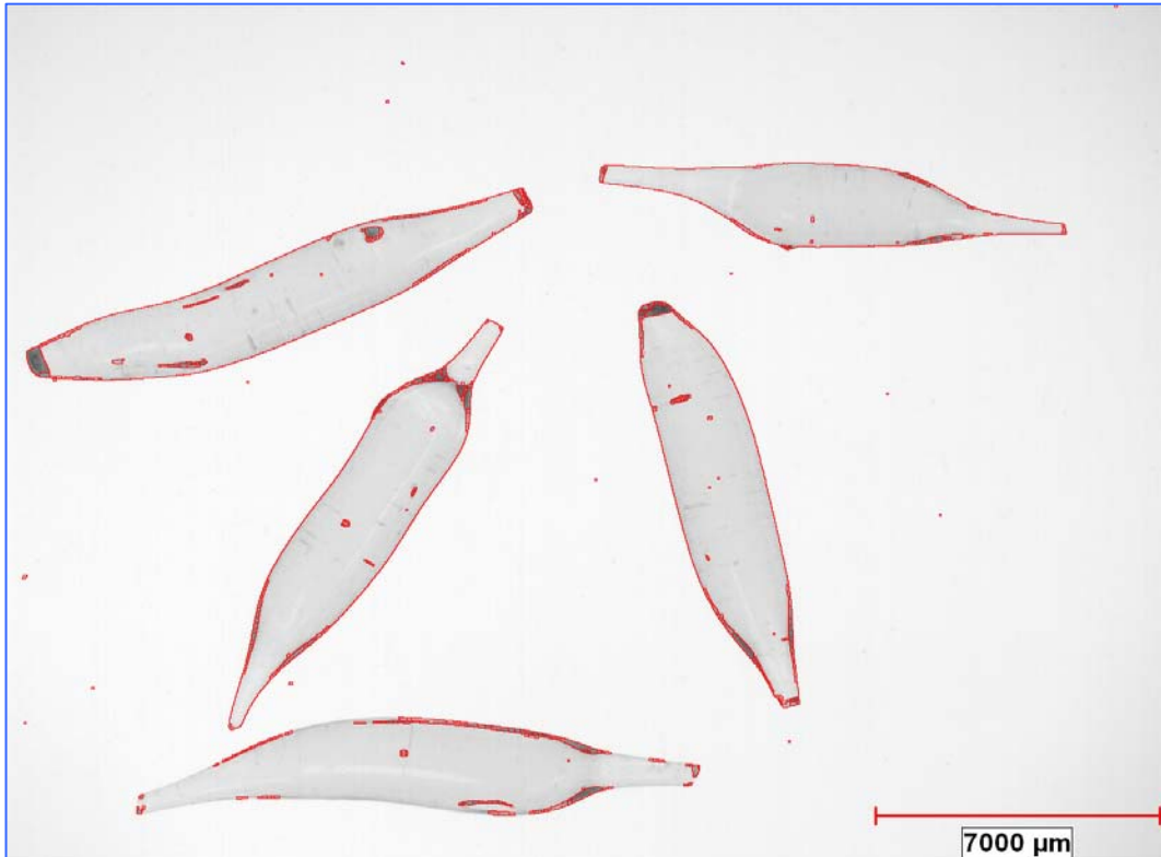
Figure 2: Defects as first detected including part of the beads outline.
